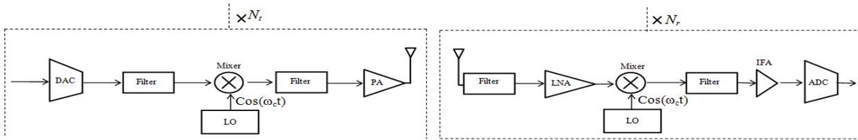
Figure 3. Transmitter and receiver architecture for WOFDM (analog).
