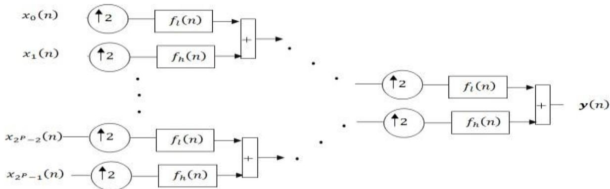
Fig 1.Symmetric multistage synthesis side QMF bank
