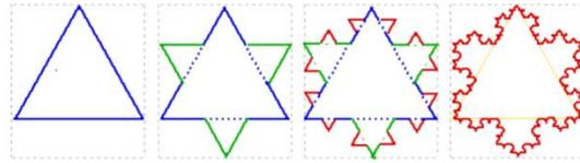
Figure 15: Iterations of Koch snowflake structures.
