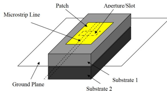
**Figure 3: Aperture coupling feed microstrip antenna**
