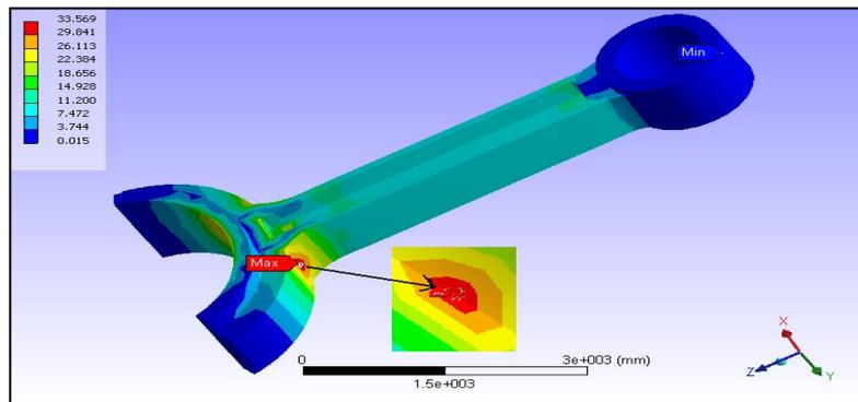
Figure 8. I section Connecting Rod Critical point
