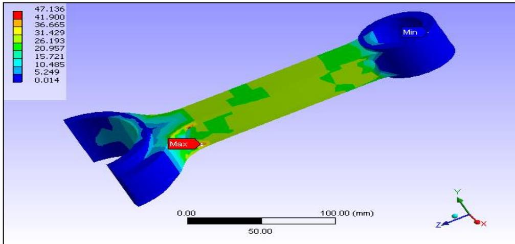
Figure 15. H section connection rod Fatigue Analysis
