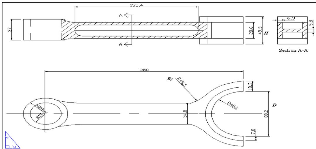
Figure 3.10: The H section connecting rod's geometry [9]
