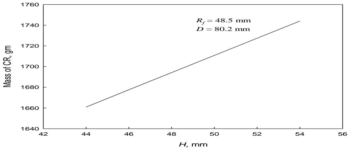
Figure 22. The effect of height ( $H$ ) of the big end on the mass of I section connecting rod, keeping other dimensions' constant
