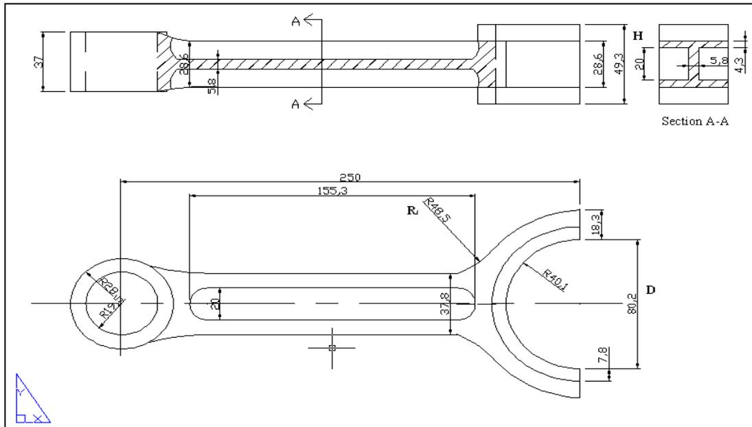
**Figure 1. The I section connecting rod's geometry**
