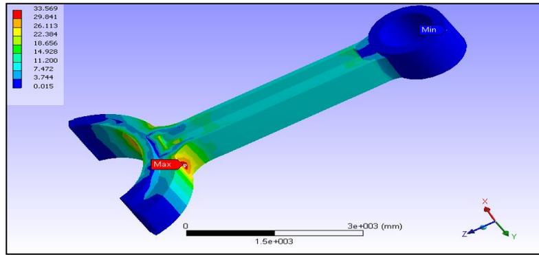
Figure 7. I section connection rod Fatigue Analysis
