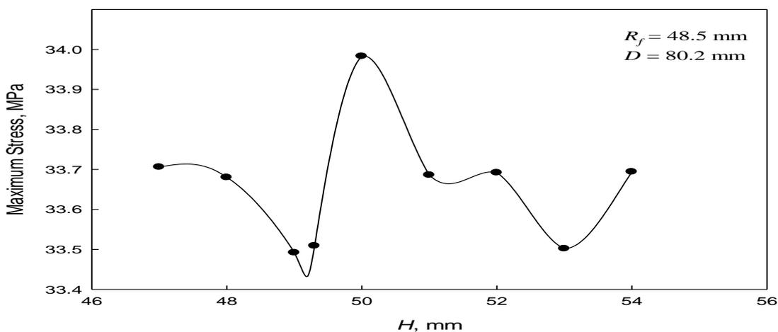
Figure 23. The effect of height ( $H$ ) of big end on the ( $\sigma_{\max}$ ) generated at the critical point, keeping other dimensions' constant
