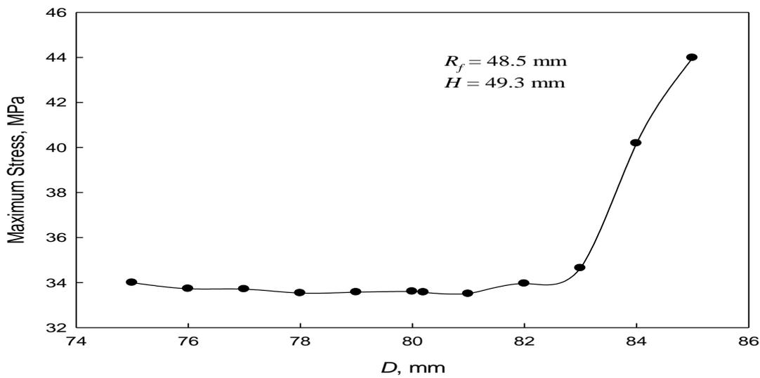
Figure 21. The effect of big end “D” on the  $(\sigma_{\max})$  generated at the critical point under the cyclic loading
