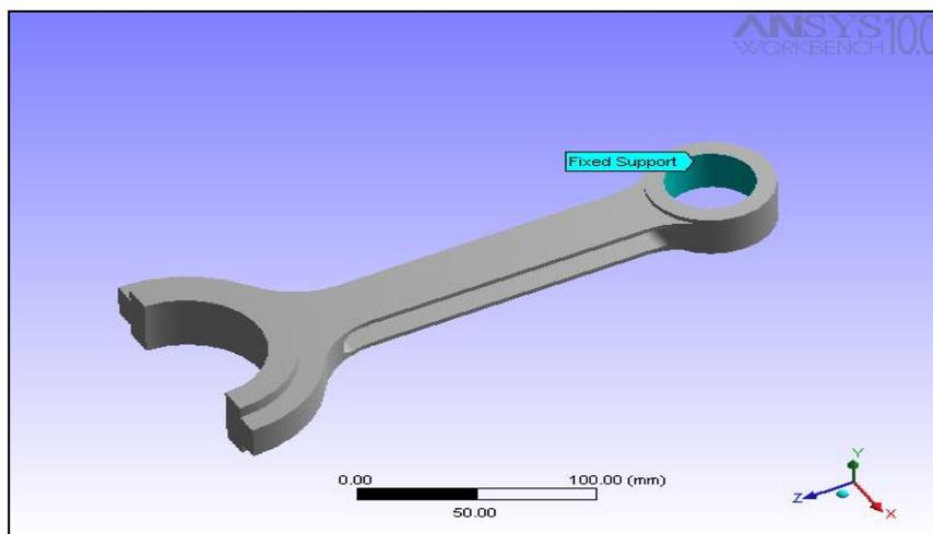
Figure 14. A model in which the small end of H section connecting rod is restrained
