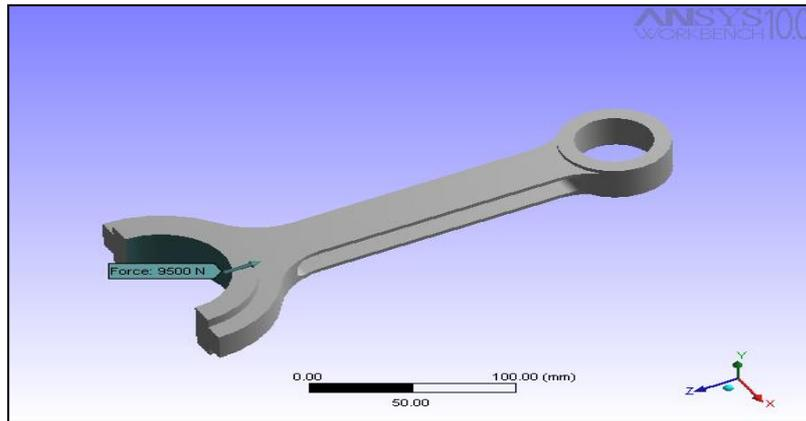
Figure 13. A sinusoidal distributed loading under tensile loading on H section connecting rod
