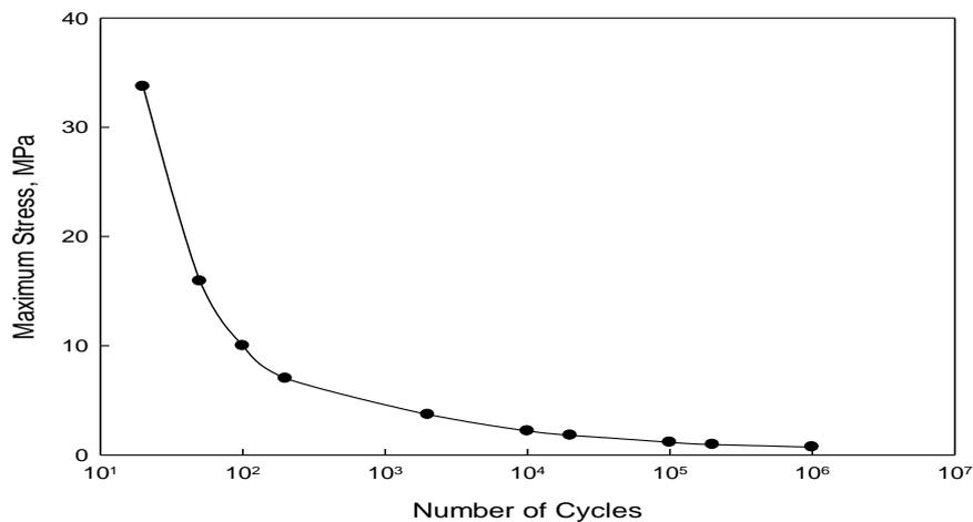
Figure 9. I section connecting rod subjected to a fatigue loading
