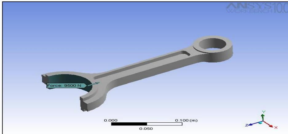
**Figure 5. A sinusoidal distributed loading under tensile loading on I section connecting rod**
