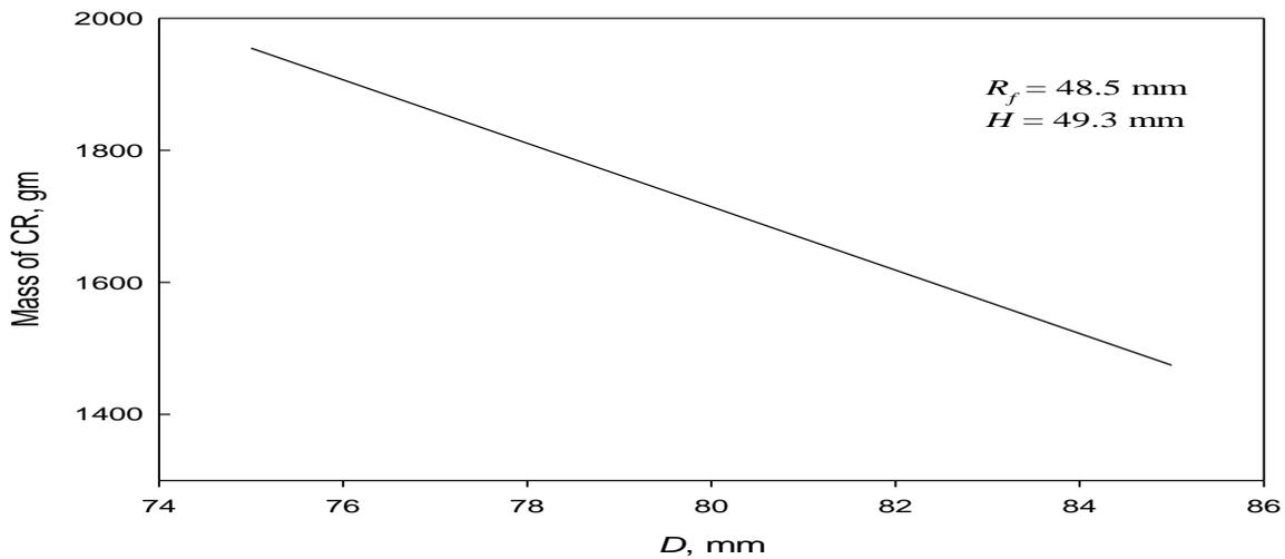
Figure 20. The effect of big end inner diameter (D) on the mass of I section connecting rod
