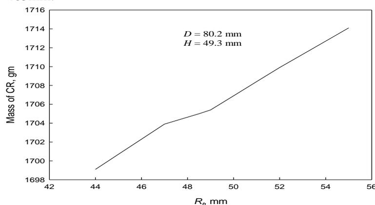
**Figure 18. The effect of fillet radius near the big end on the mass of I section connecting rod**
