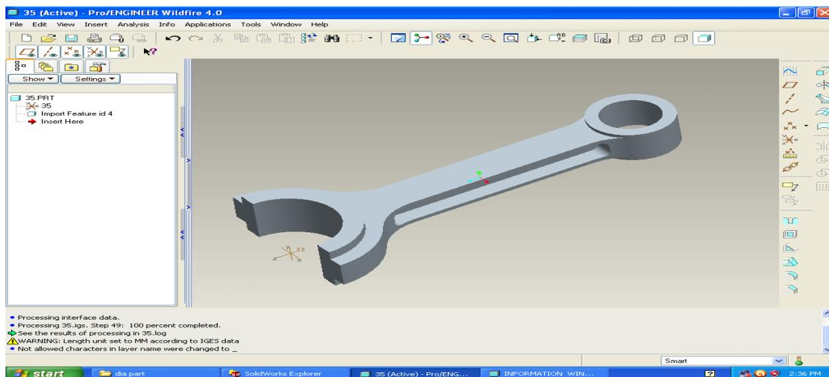
Figure 11. Geometrical Model of H Section Connecting Rod
