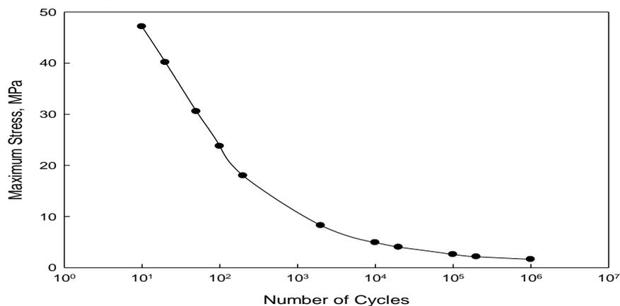
Figure 17. H section connecting rod subjected to a fatigue loading
