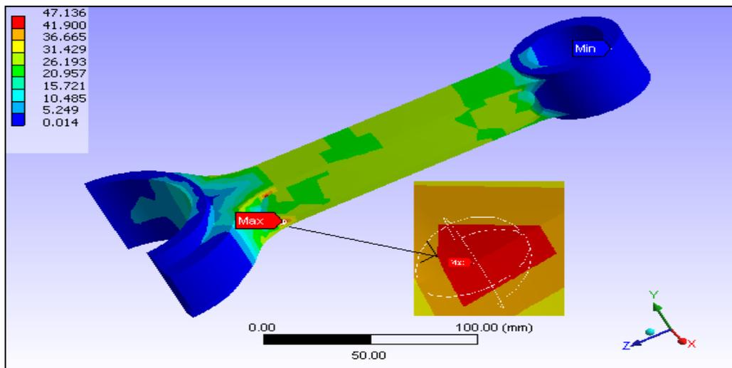
Figure 16. H section Connecting Rod Critical point
