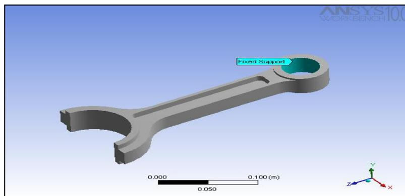
**Figure 6. The small end of I section connecting rod**
