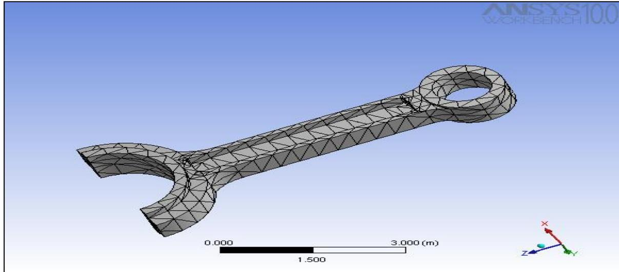
Figure 3. I section Connecting Rod Meshing Model
