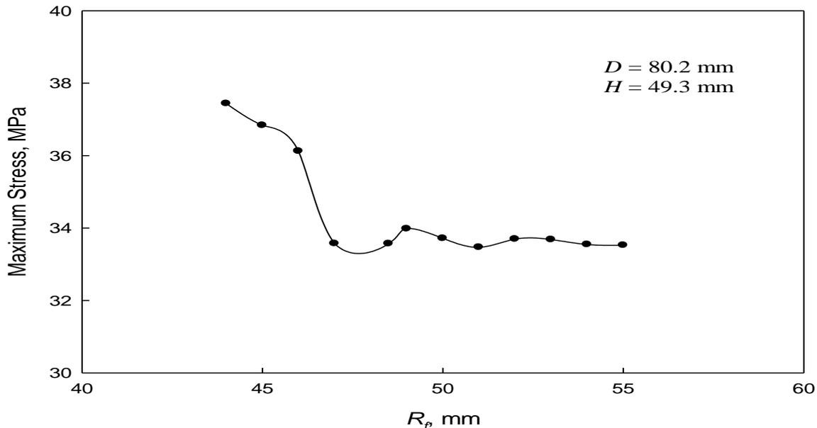
**Figure 4.2: Maximum stresses produced at the critical point during cyclic loading and the impact of large end fillet radius**
