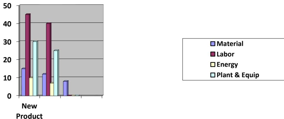
This chart illustrates conservation of value in a product that is remanufactured versus one that is recycled. The relative costs of material, labour, energy and the contribution of plant and equipment to a product in its manufacture are shown on the left. Remanufacturing preserves much of this value while adding a second life to the product. In contrast, recycling shreds the product in an attempt to
