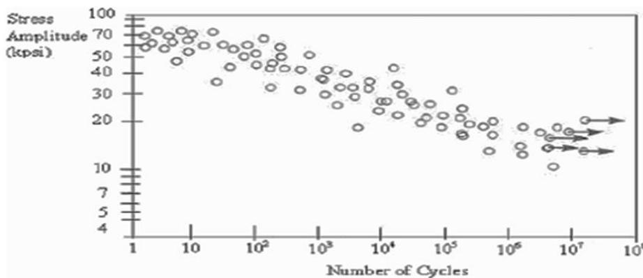
Figure 11. A typical S-N material data [25]
