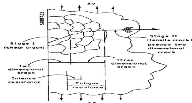
Figure 9 The transition form of crack growth. [29]
