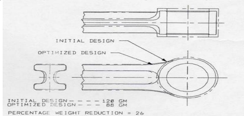
**Figure 1. Final and initial designs for the wrist pin end of a connecting rod [21]**
