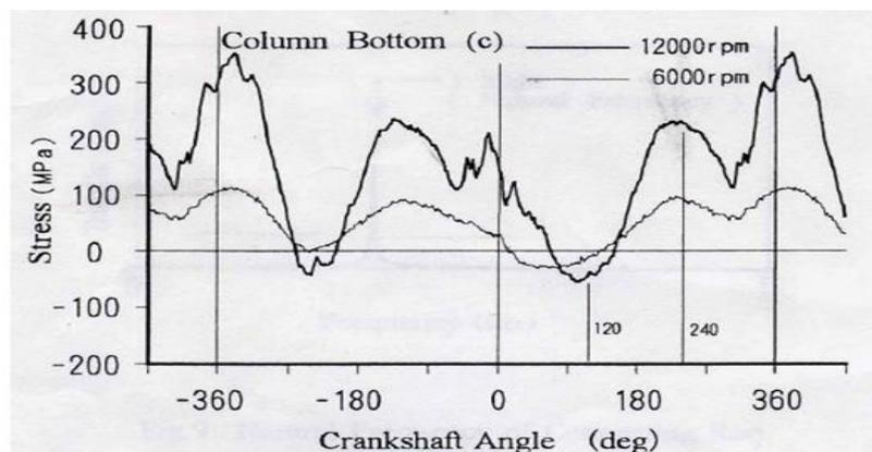
**Figure 4. Stresses at the bottom of the connecting rod column [27]**
