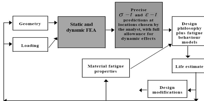
Figure 19 A View of Life Estimation Procedure Using Finite Element Analysis [29]
