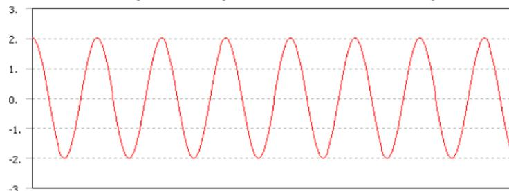
Figure 6. A constant amplitude loading [28]
