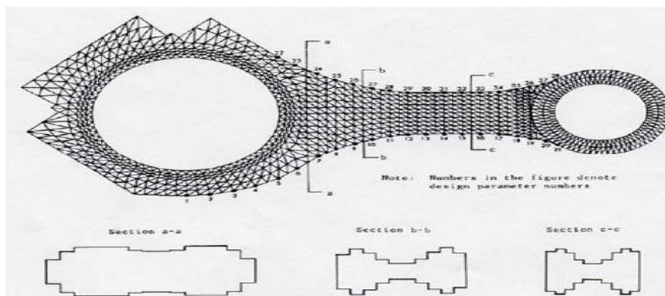
**Figure 2. The optimum design obtained [22]**
