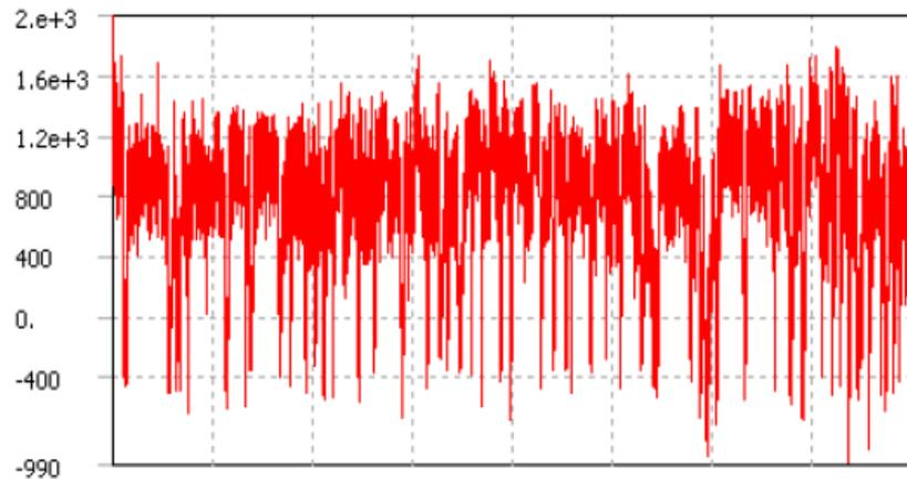
Figure 7. A constant amplitude, non-proportional loading [28]
