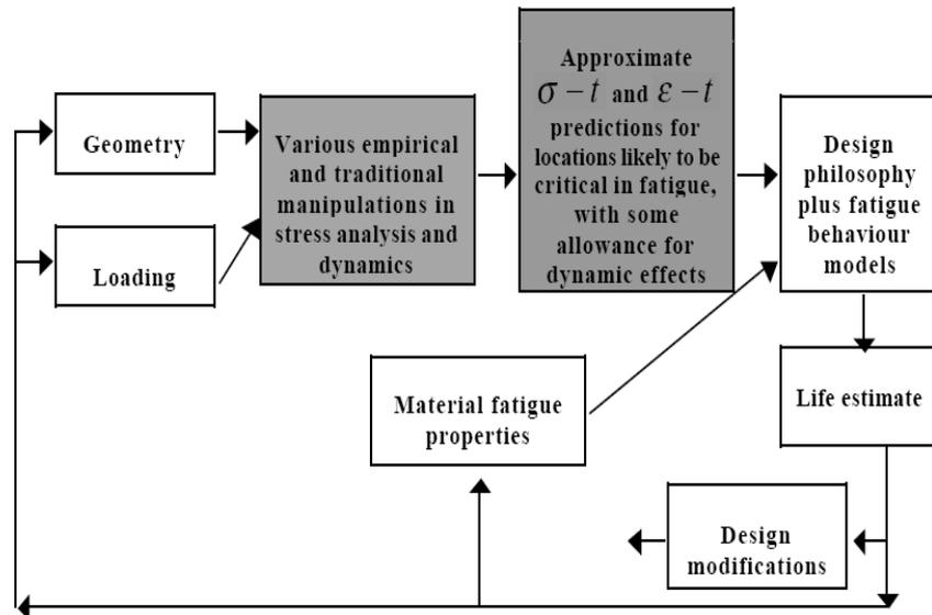
Figure 18. A View of Traditional Life Estimation Procedure [29]
