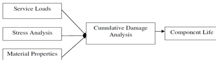
**Figure 13. The cumulative damage analysis process [30]**
