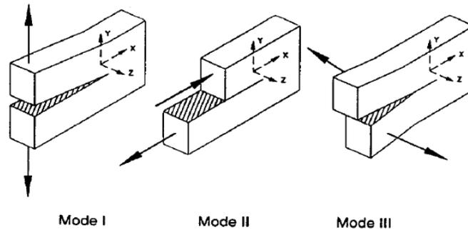
Figure 8. The three cracking modes that fracture mechanics uses. [29]
