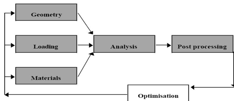
**Figure 17. A Conventional View of Fatigue Analysis Process [29]**
