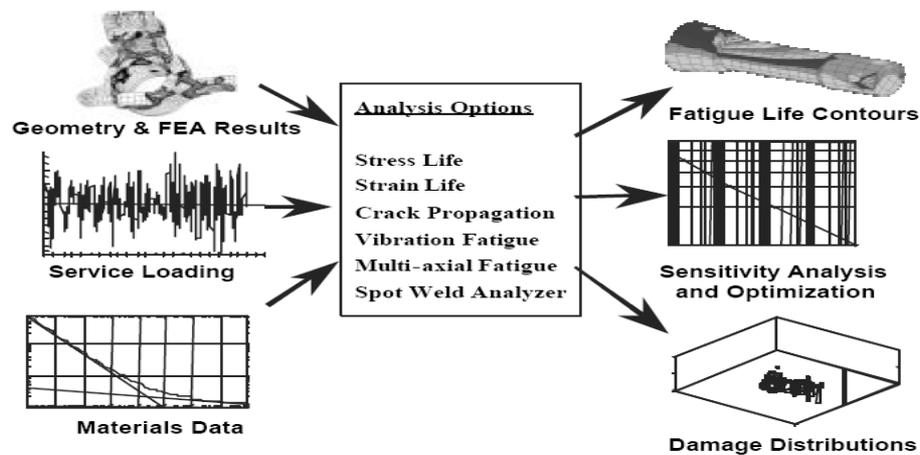
**Figure 2.15: An overview of the Finite Element Analysis based fatigue environment [29]**
