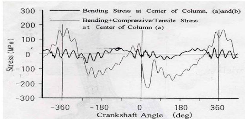
Figure 5. Stresses at the centre of the connecting rod column [27]
