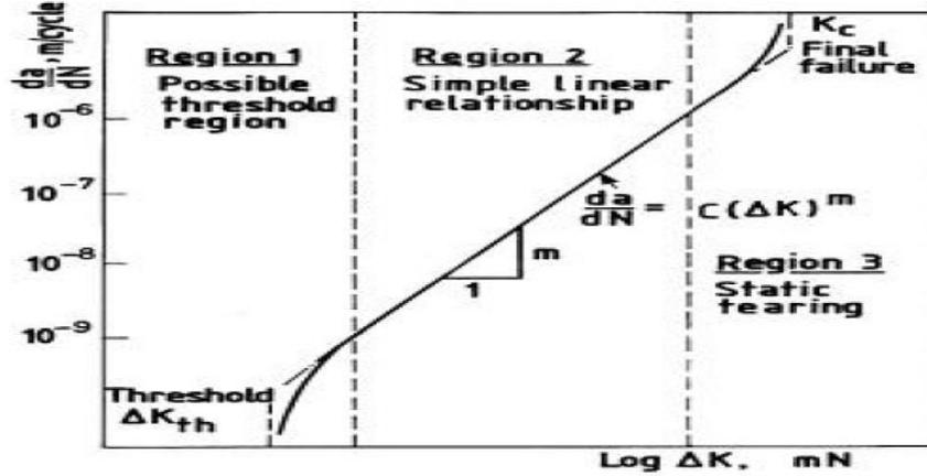
Figure 10. Crack Propagation Rate at constant  $\Delta K$ . [29]
