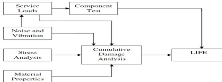
**Figure 12. The fundamental components of fatigue design methodology [30]**
