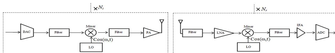
**Figure 3.** Transmitter and receiver architecture for WOFDM (analog).
