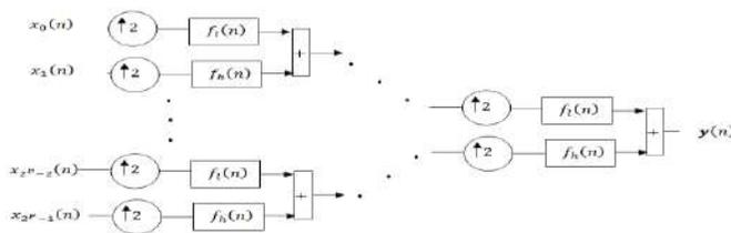
**Figure 1.** Symmetric multistage synthesis side QMF bank
