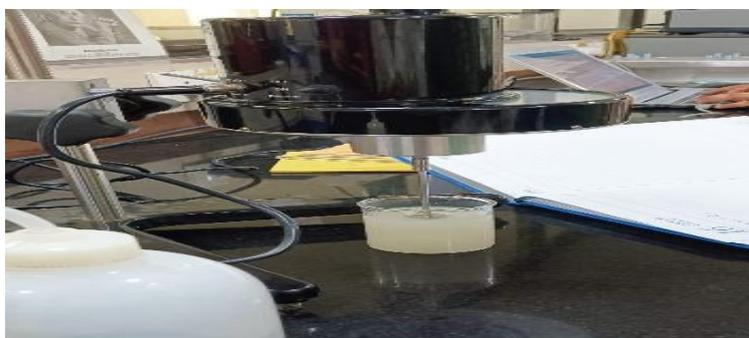
**Figure No 3: Viscosity determination by Brookfield viscometer**
